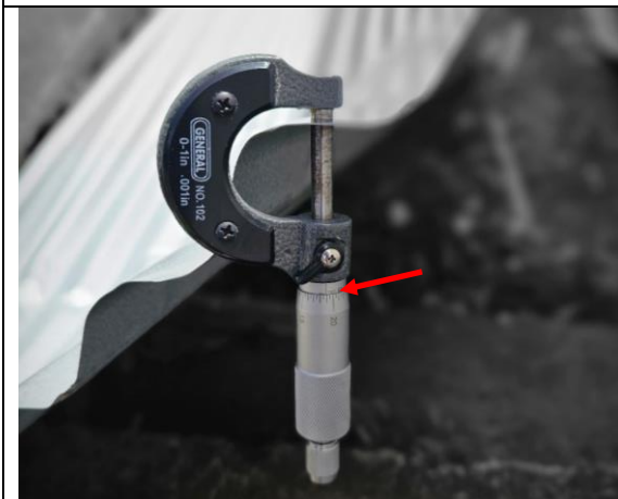
Metal thickness measured at 0.019” (0.48 mm), including the zinc finish.
